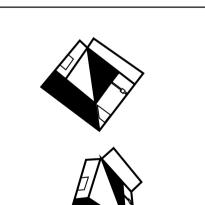
Fix nose cone (part 2) onto cylinder (part 1), by glueing the tabs on the end of part 1, and inside edge of part 2. Bend the tabs inwards slightly before attaching the nose cone.  Fold the fins (parts 3–6) diagonally into triangles, and fold tabs outwards 90°.
