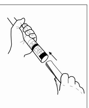
3. Insert a piece of rolled up paper into the cylinder for extra stability and to aid fixture of the nose cone.
