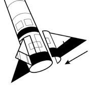
6. Glue the fins into position at the bottom of the rocket, matching the design on the tabs to the design on the rocket body.
